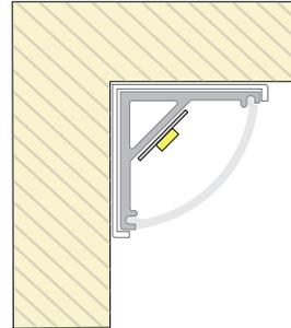
The Surfa 2 is ideal for general low-profile corner mounting of LED tape light so that it shines at a 45 degree angle from the surface. Surfa 2 corner connectors can be used to link channel section seamlessly around corners, while straight connectors can join straight sections of channel for longer runs. Surfa 2 is perfect for directional lighting.
